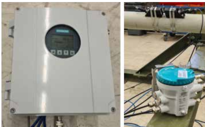
Figure 7: Wide-Beam Sensors F55200 in 2-path reflect mount, FS230 transmitter and External DSL
